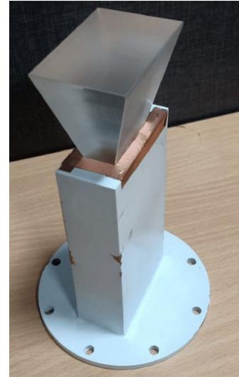
**FIGURE 18.** Fabricated antenna with tapered transition as in [15].
