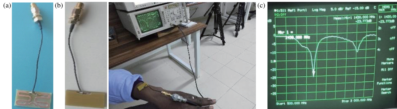
FIGURE 7. Measurement: (a) antenna prototype, (b) experimental setup, (c) reflection coefficient on benign tissue.
