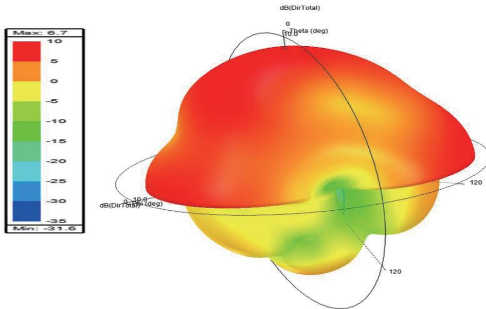
**FIGURE 4.** 3D proposed antenna's radiation far-field pattern.
