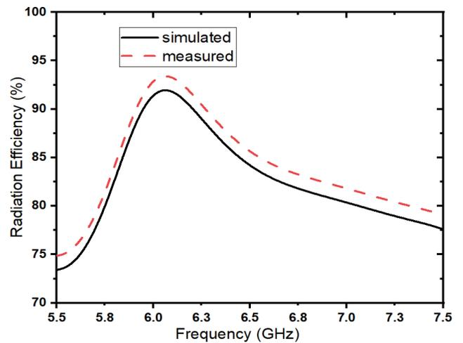
FIGURE 13. Radiation efficiency versus Frequency.
