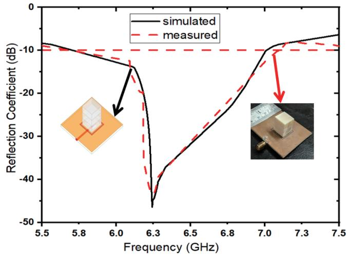
FIGURE 8. Reflection coefficient versus frequency.
