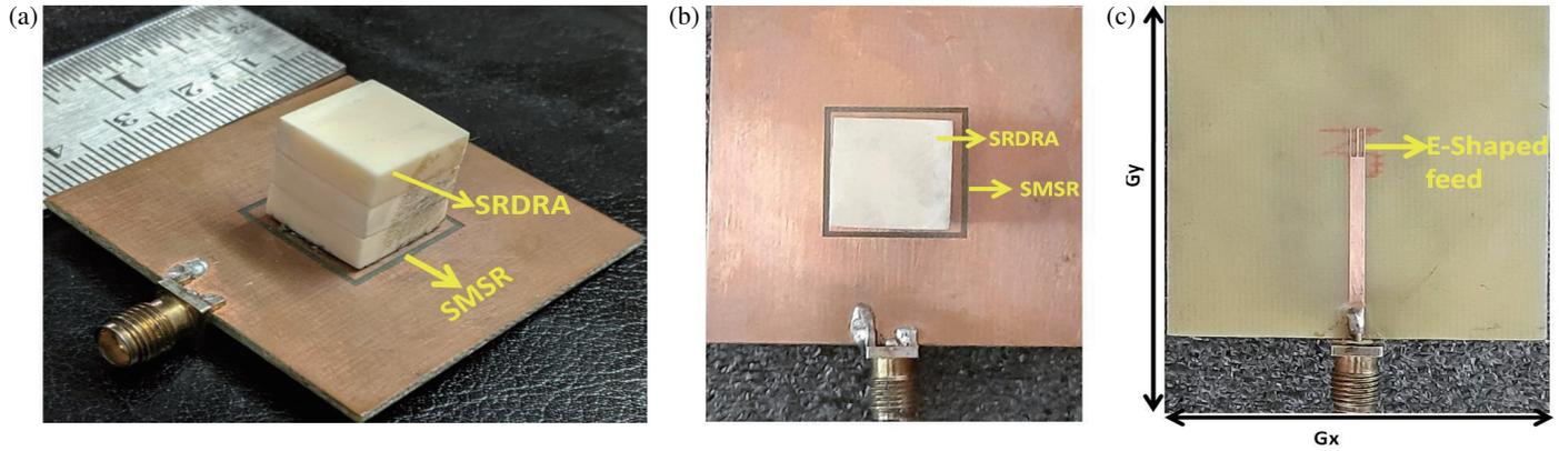
FIGURE 5. (a). 3D view of proposed antenna. (b) Top view with SMSR and SRDRA. (c) Bottom view with E-shaped microstrip feed.
