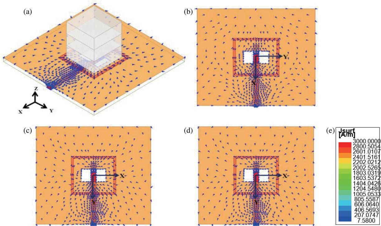
**FIGURE 3.** Antenna current distribution on surface. (a) 3D view (XYZ)  $\Phi = 0^\circ$ . (b) Top View (XY)  $\Phi = 90^\circ$ . (c) Top view (XY)  $\Phi = 180^\circ$ . (d) Top view (XY)  $\Phi = 270^\circ$ . (e) Scale for a, b, c & d at 6.2 GHz.
