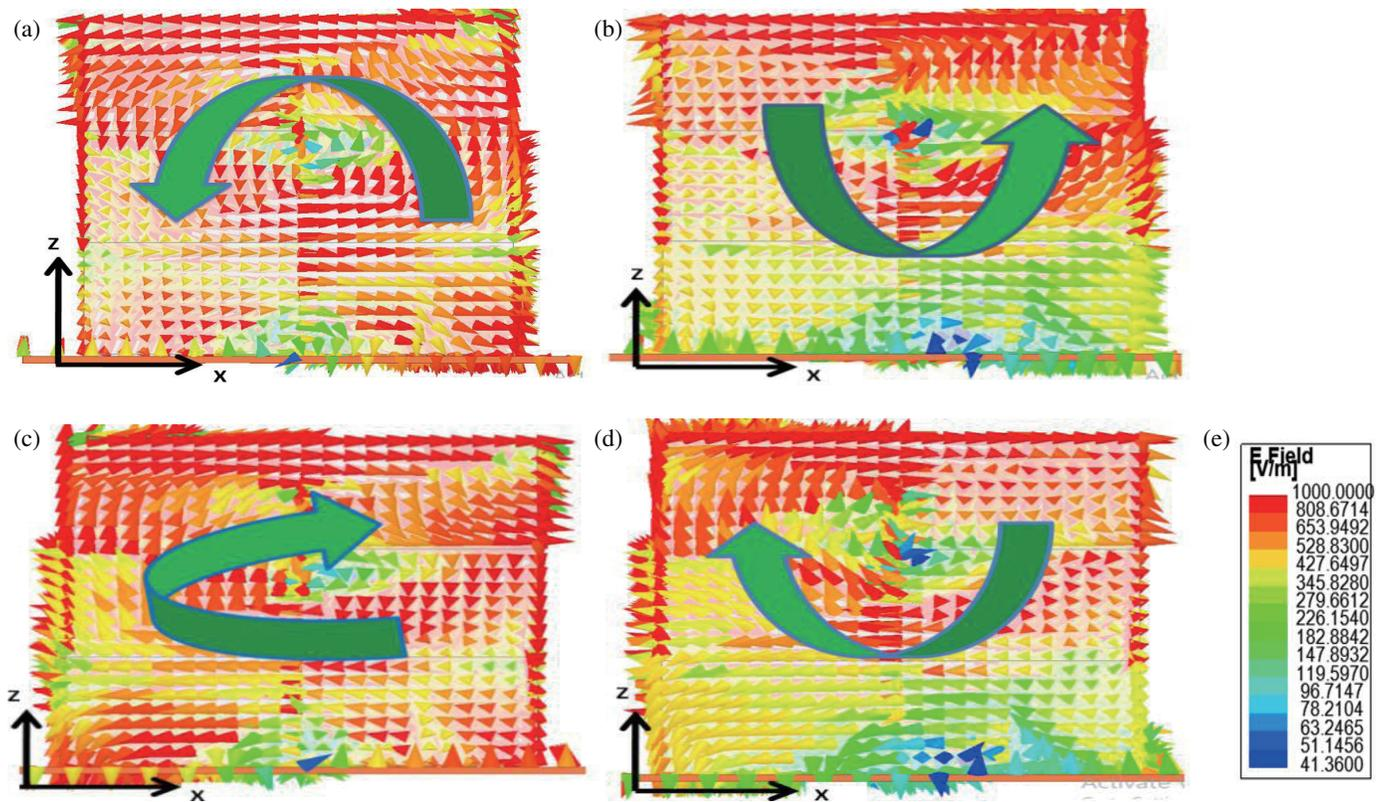
**FIGURE 2.** Left side view of the Antenna  $E$ -field distribution (a)  $\Phi = 0^\circ$  (b)  $\Phi = 90^\circ$  (c)  $\Phi = 180^\circ$  (d)  $\Phi = 270^\circ$  (e) Scale for a, b, c & d at 6.2 GHz.
