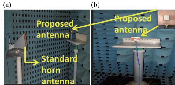
FIGURE 7. Gain and far-field measurements set up with SRMSR DRA (a) & (b).
