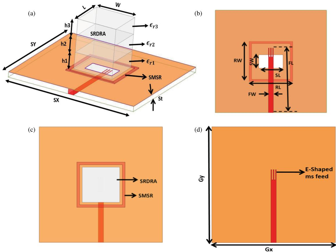
**FIGURE 1.** The Geometry of the proposed Antenna. (a) Isometric view. (b) Top view without SRDRA with aperture slot. (c) Top view SRDRA with SMSR. (d) Bottom view with E-shaped microstrip feed.
