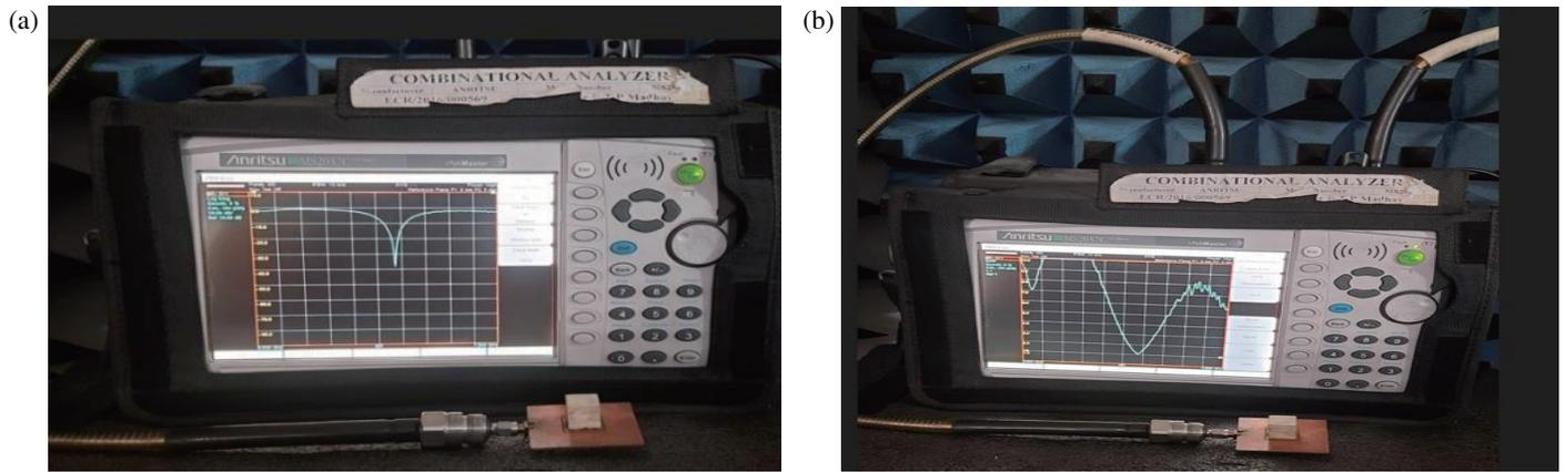
FIGURE 6. SRSMSRDRA. (a) Reflection coefficient measurement setup. (b) Measurement setup VSWR.
