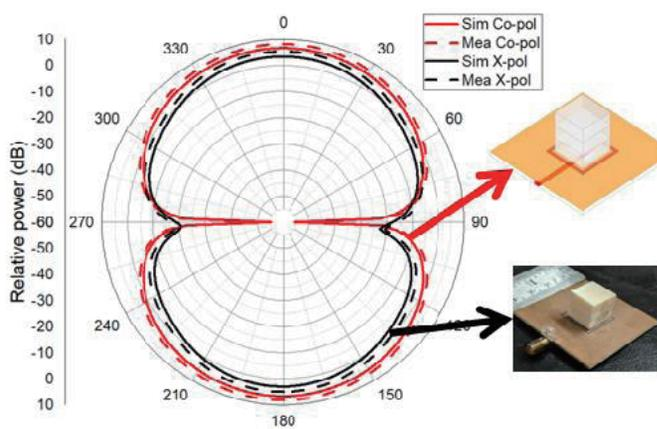
FIGURE 10. 2D radiation pattern (*E*-plane).
