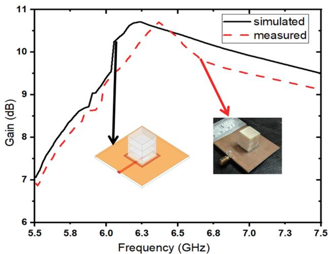
FIGURE 12. Gain versus Frequency.
