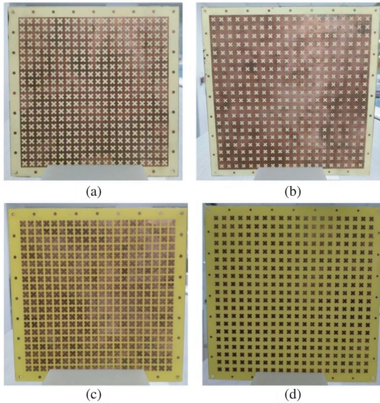
**Figure 13.**  $20 \times 20$  arrangement of the unit cells: (a) slot array layer for  $L = 5.5$  mm, (b) slot array layer for  $L = 8$  mm, (c) patch array layer for  $L = 5.5$  mm and (d) patch array layer for  $L = 8$  mm.
