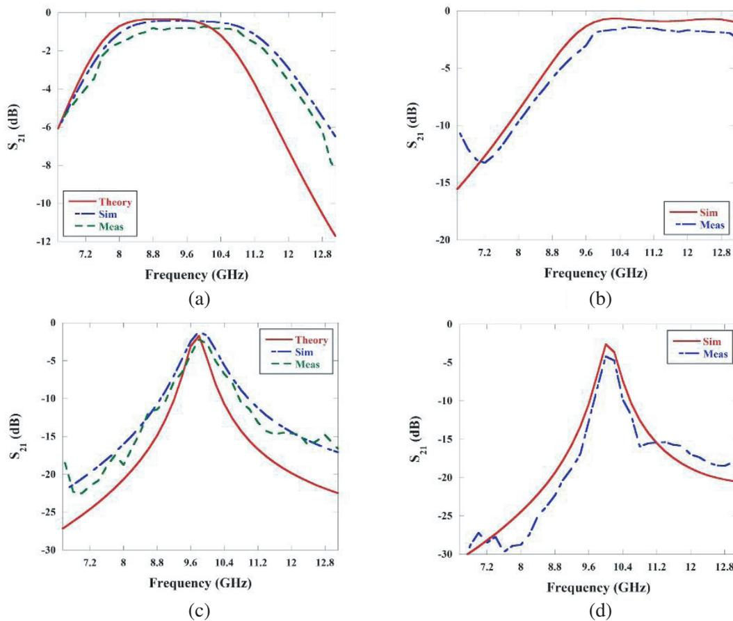
**Figure 15.** Result comparison for the fabricated prototypes viz. (a) PSP (unit cell periodicity = 5.5 mm, substrate thickness = 1.6 mm), (b) PSP (unit cell periodicity = 8 mm, substrate thickness = 1.6 mm), (c) SPS (unit cell periodicity = 5.5 mm, substrate thickness = 0.8 mm) and (d) SPS (unit cell periodicity = 8 mm, substrate thickness = 0.8 mm) configurations against theory and simulations.
