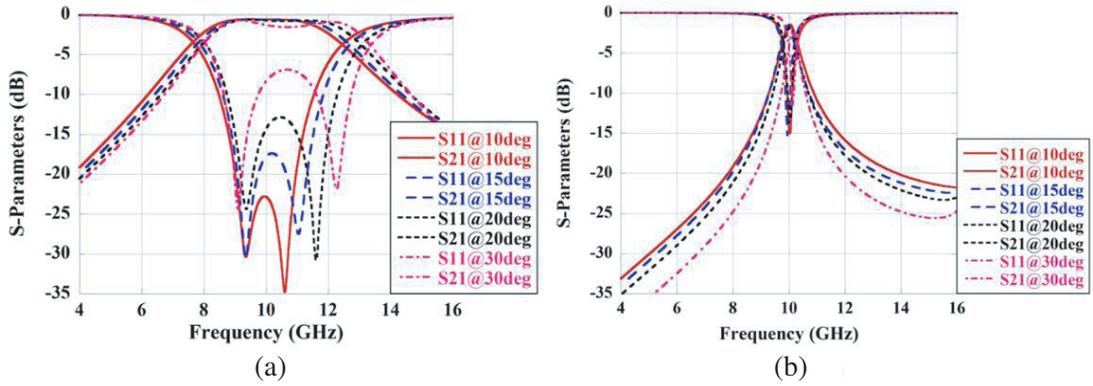
**Figure 11.** Oblique incidence performance for the (a) PSP (unit cell periodicity = 5.5 mm, substrate thickness = 1.6 mm) and (b) SPS (unit cell periodicity = 5.5 mm, substrate thickness = 0.8 mm) configurations respectively.
