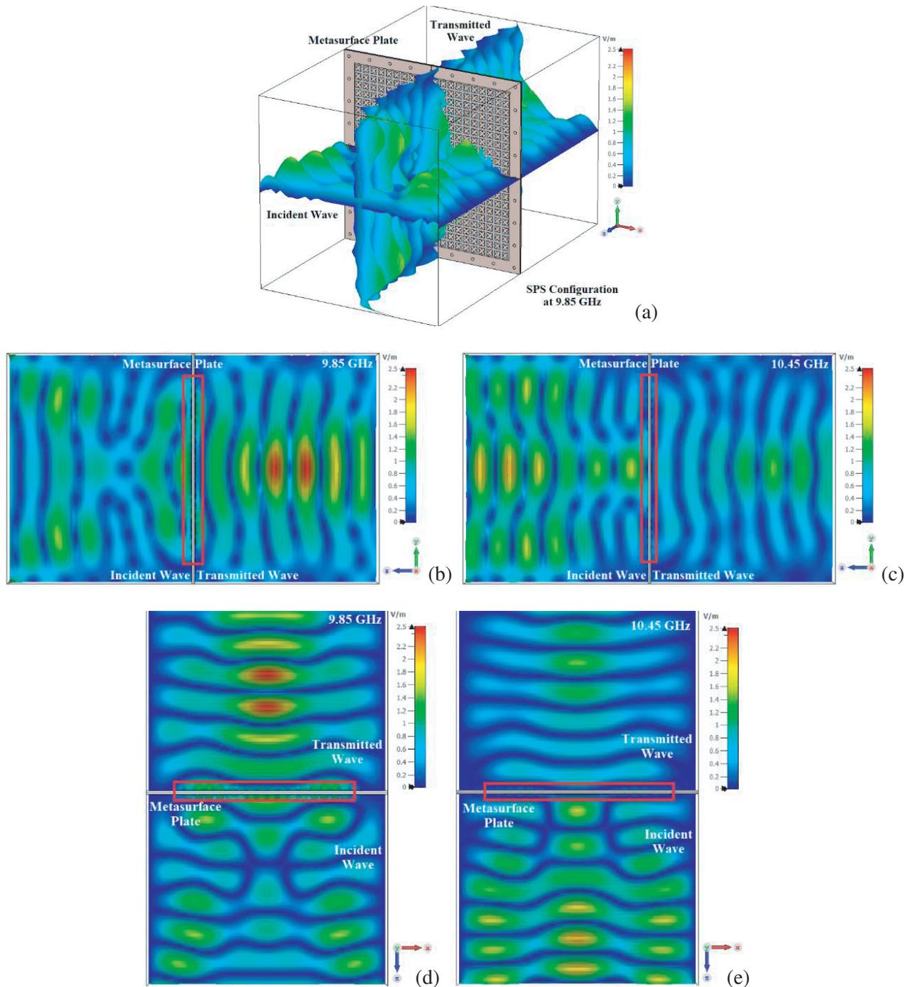
**Figure 12.** (a) Perspective view of the simulation setup with the metasurface being excited by a plane wave source, (b) *E*-field propagation along *YZ* plane at 9.85 GHz and (c) 10.45 GHz, (d) *E*-field propagation along *XZ* plane at 9.85 GHz and (e) 10.45 GHz.
