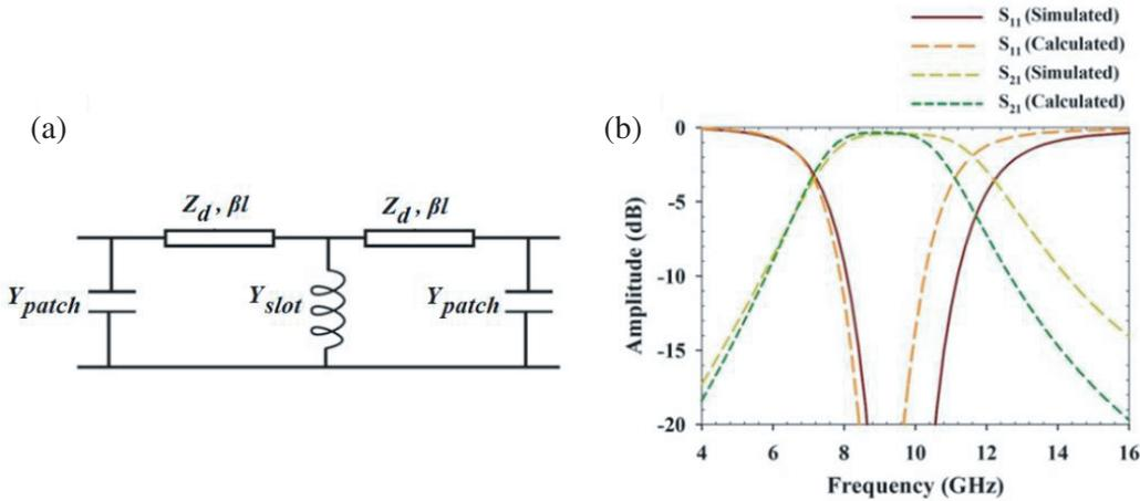
**Figure 8.** (a) Equivalent circuit model of the Patch-Slot-Patch (PSP) configuration and (b) comparison between the theoretical and simulated  $S$ -parameter results calculated at unit cell periodicity of  $L = 5.5$  mm,  $A = 4$  mm,  $h = 1.6$  mm.
