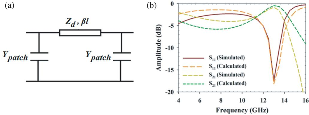
**Figure 5.** (a) Equivalent circuit model of the Patch-Substrate-Patch configuration shown in Fig. 3, and (b) comparison between the theoretical and simulated  $S$ -parameter results, for  $A = 4$  mm,  $L = 5.5$  mm, and  $h = 1.6$  mm respectively.
