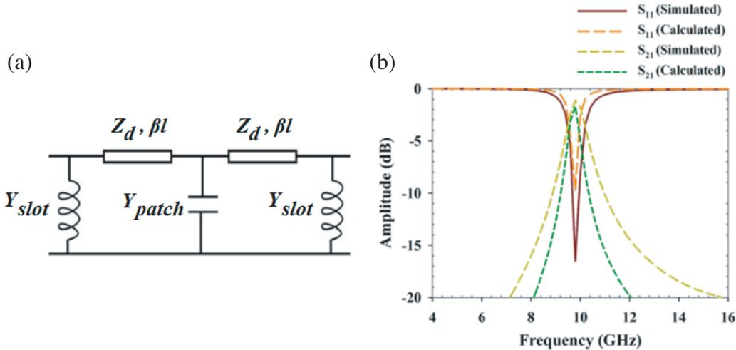
**Figure 10.** (a) Equivalent circuit model of the Slot-Patch-Slot (SPS) configuration and (b) comparison between the theoretical and simulated  $S$ -parameter results calculated at unit cell periodicity of  $L = 5.5$  mm,  $A = 4$  mm,  $h = 0.8$  mm.
