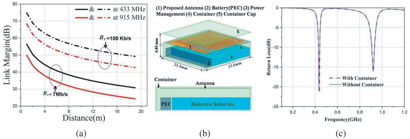
**Figure 7.** (a) Link margin. (b) An expansive outlook of the wearable system. (c) Return loss of the proposed antenna.
