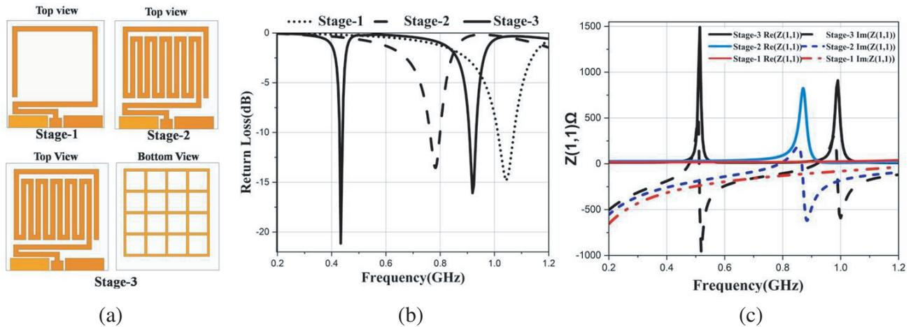
**Figure 2.** (a) Developmental stages of proposed design. (b) Return Loss plot from stage 1 to stage 3. (c) Impedance plot from stage 3 to stage 1.
