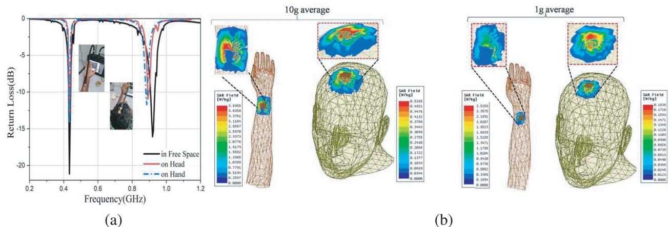
**Figure 6.** Assessment of Antenna SAR using a human body model. (a) Comparative analysis of return loss: Free space vs. hand and head positions. (b) Three-dimensional SAR distribution of antenna at 433 MHz on hand and head position.
