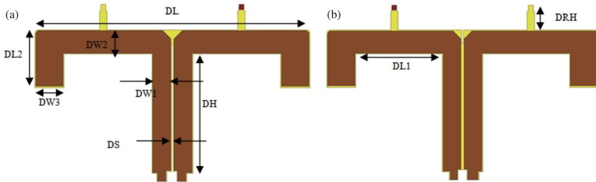
FIGURE 2. (a) Dipole 1 and (b) Dipole 2.
