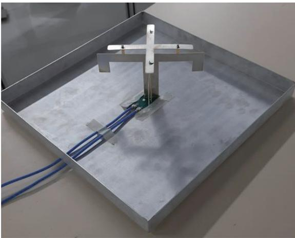
**FIGURE 5.** Photograph of the fabricated antenna.
