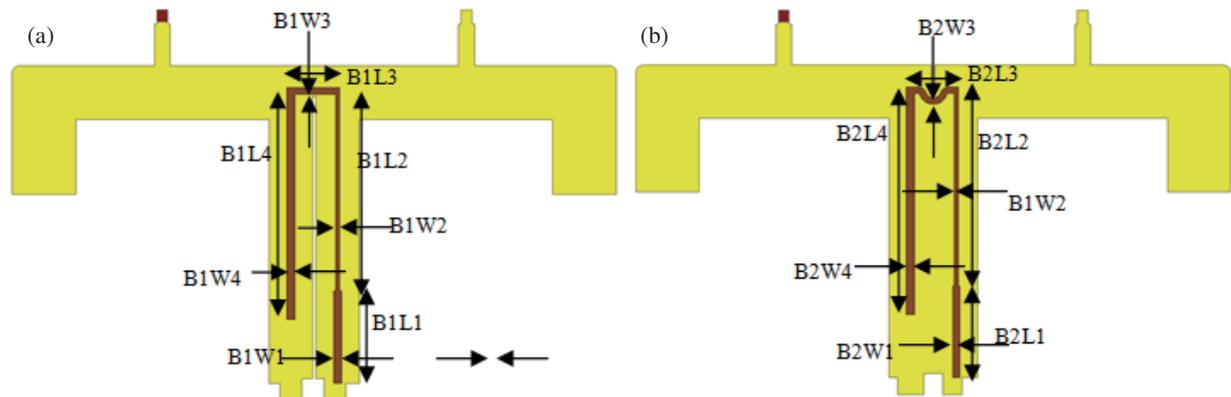
FIGURE 3. (a) Dipole 1 Balun and (b) Dipole 2 Balun.
