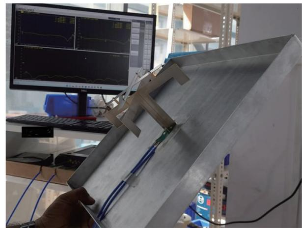
**FIGURE 6.** Measurement setup of the fabricated antenna.
