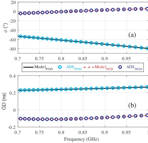
**Figure 8.** Comparison of PGD and NGD (a) phase, and (b) GD from modelling and ADS<sup>®</sup> simulation.
