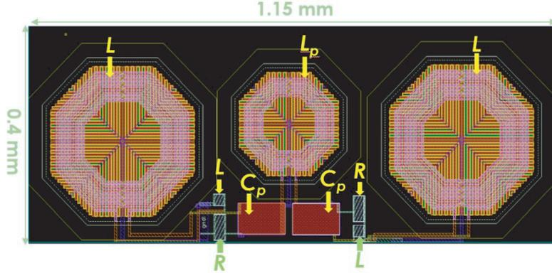
**Figure 7.** Layout design of miniature CPS IC in the Cadence VIRTUOSO<sup>®</sup> environment.
