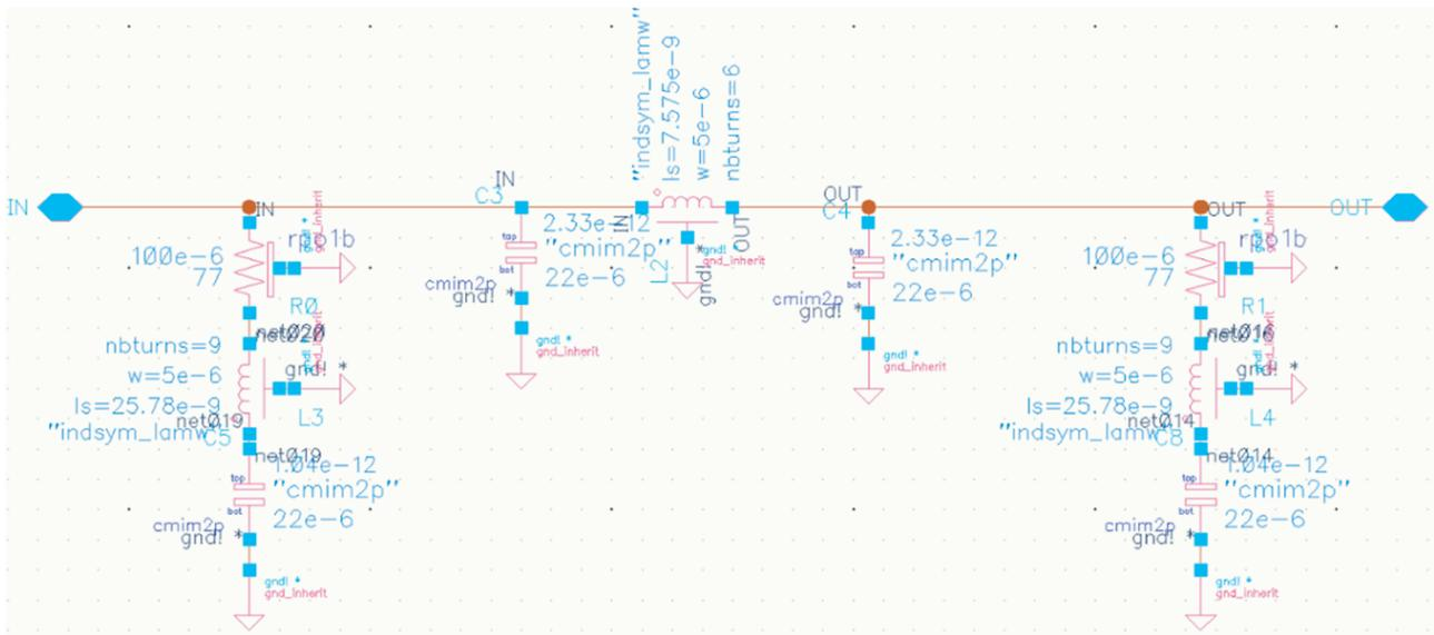
**Figure 6.** Schematic design of CPS IC in the Cadence VIRTUOSO<sup>®</sup> environment.
