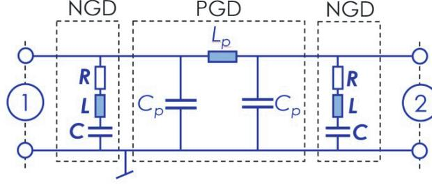
**Figure 4.** Lumped passive circuit of CPS topology.
