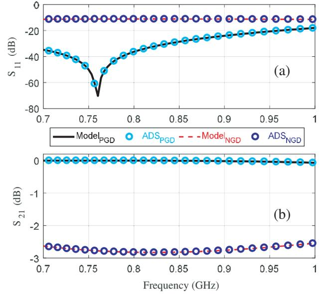
**Figure 9.** Comparison of PGD and NGD (a)  $S_{11}$  and (b)  $S_{21}$  from modelling and ADS<sup>®</sup> simulation.
