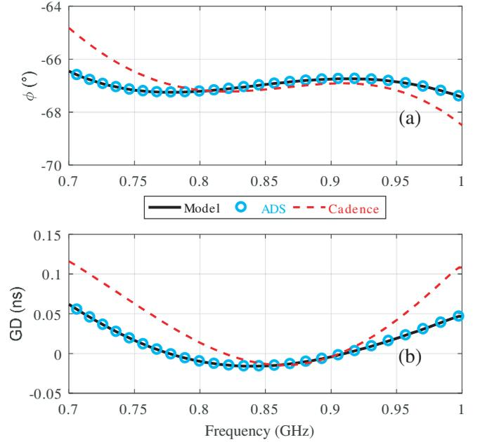
**Figure 11.** Comparison of CPS (a) phase and (b) GD from modelling, and ADS<sup>®</sup> and Cadence VIRTUOSO<sup>®</sup> simulation.
