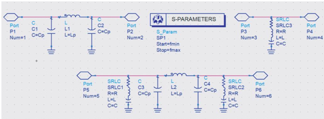
**Figure 5.** ADS<sup>®</sup> schematic design of PGD, NGD and CPS POCs.
