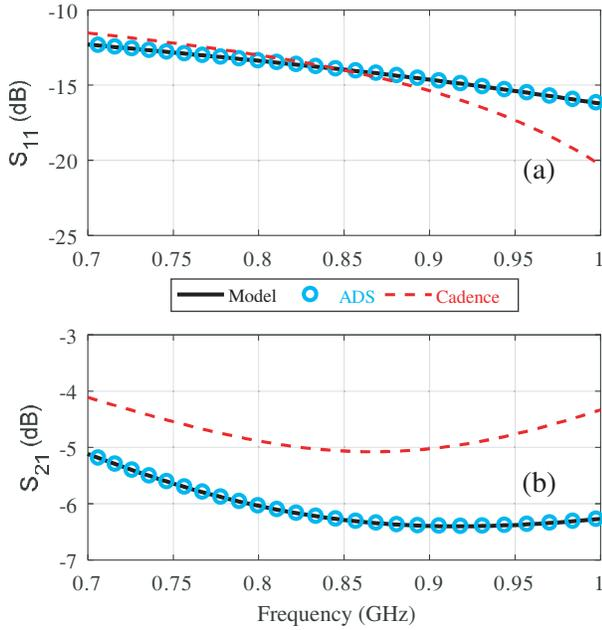
**Figure 10.** Comparison of CPS (a)  $S_{11}$  and (b)  $S_{21}$  from modelling, and ADS<sup>®</sup> and Cadence VIRTUOSO<sup>®</sup> simulations.
