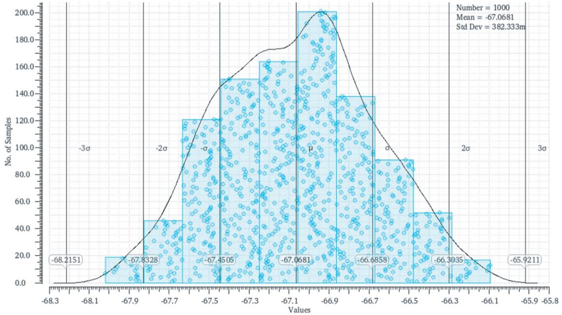
Figure 12. Histogram of CPS IC layout  $\varphi_0$  from MC analysis.
