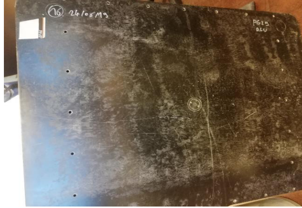
Figure 1. Photo of composite 1 (120 cm × 90 cm × 2.6 mm).
