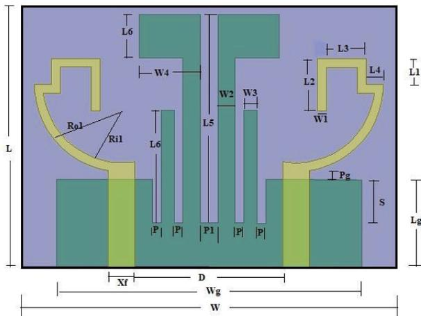
**Figure 1.** Geometry of the antenna.
