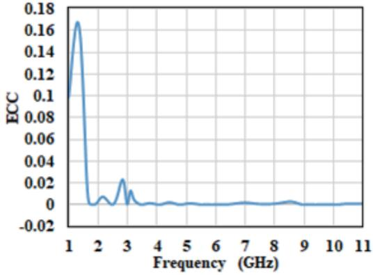
Figure 9. ECC of antenna.
