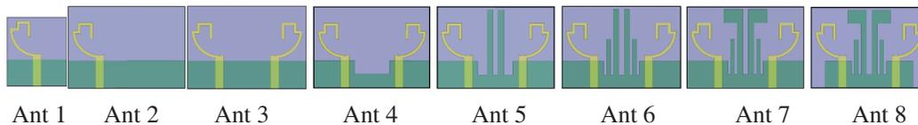
**Figure 3.** Evolution stages of antenna.
