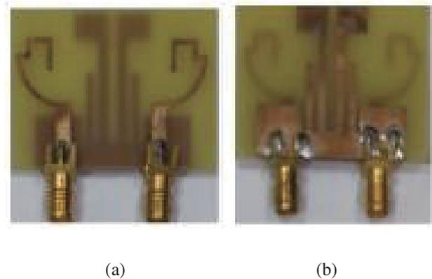
**Figure 2.** Fabricated prototype antenna. (a) Top view. (b) Bottom view.
