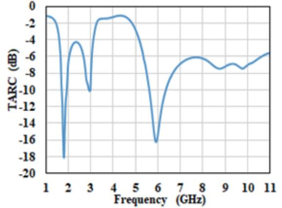
Figure 12. TARC of antenna.
