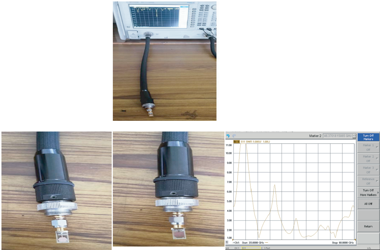
Figure 15. Measurement setup and results for VSWR parameter of the fabricated antenna.
