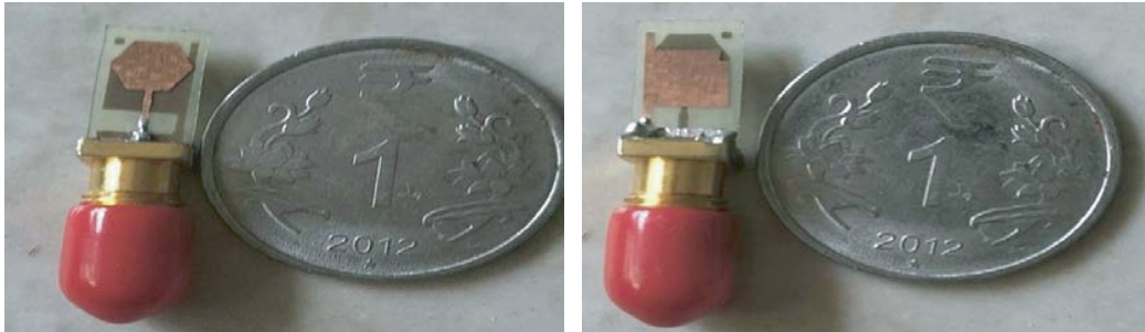
Figure 3. Hexagonal antenna of dimension 9 mm \times 5 mm. Top and Back view.
