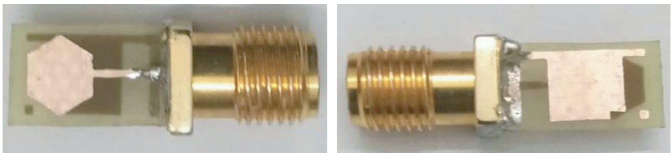
Figure 14. Fabricated antenna top and bottom views.
