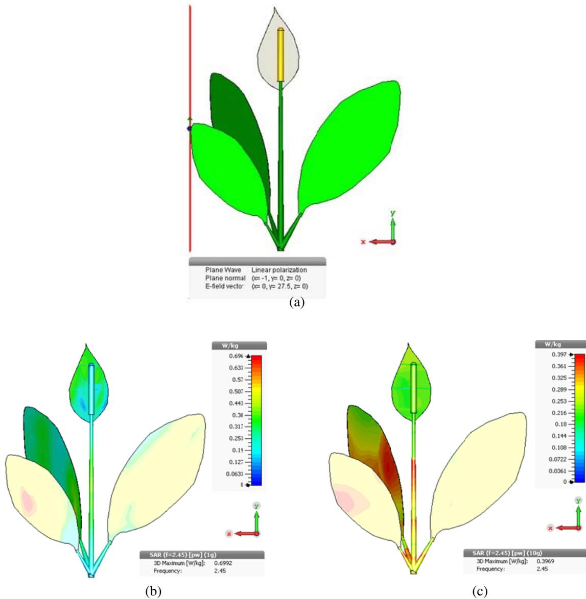
**Figure 3.** (a) A linearly polarized plane wave has impinged on the Peace Lily model with Direction of Propagation (DoP):  $x = -1$  and  $E$  field:  $y$  axis, (b) corresponding 1 g spatial SAR distribution at 2450 MHz and (c) corresponding 10 g spatial SAR distribution at 2450 MHz.
