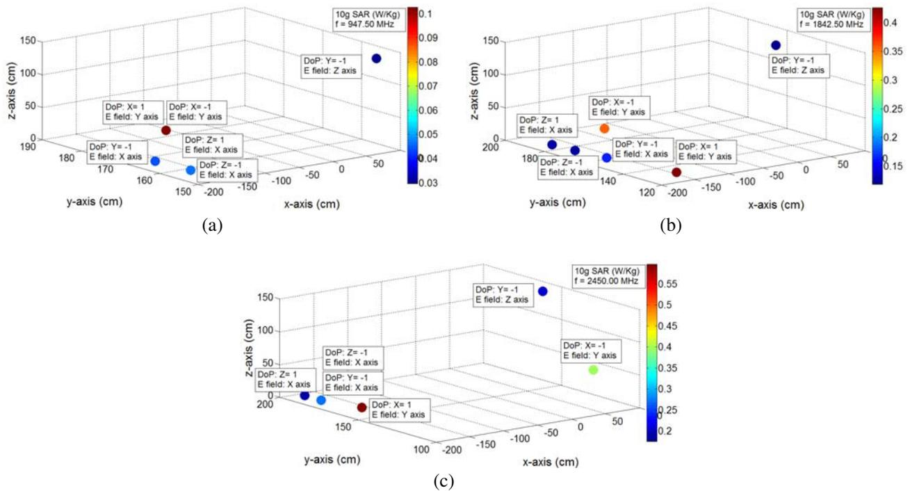
**Figure 6.** (a) to (c) Contrasts in magnitude and spatial coordinates of 10 g averaged SAR for six distinct combinations of direction of arrival and polarization of incident wave at 947.50 MHz, 1842.50 MHz and 2450 MHz.
