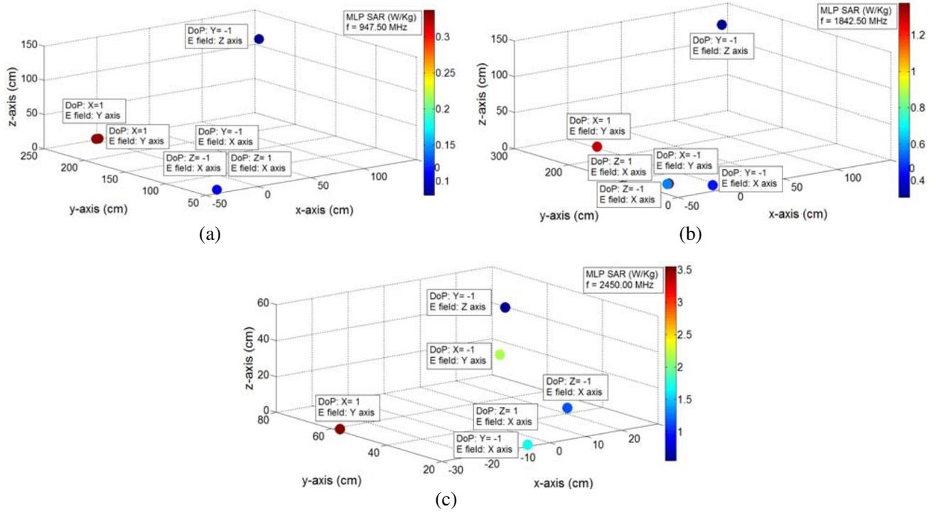
**Figure 4.** (a) to (c) Contrasts in magnitude and spatial coordinates of MLP SAR for six distinct combinations of direction of arrival and polarization of incident wave at 947.50 MHz, 1842.50 MHz and 2450 MHz.
