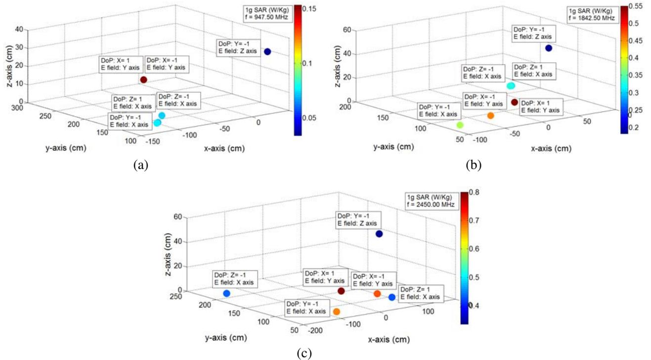
**Figure 5.** (a) to (c) Contrasts in magnitude and spatial coordinates of 1 g averaged SAR for six distinct combinations of direction of arrival and polarization of incident wave at 947.50 MHz, 1842.50 MHz and 2450 MHz.
