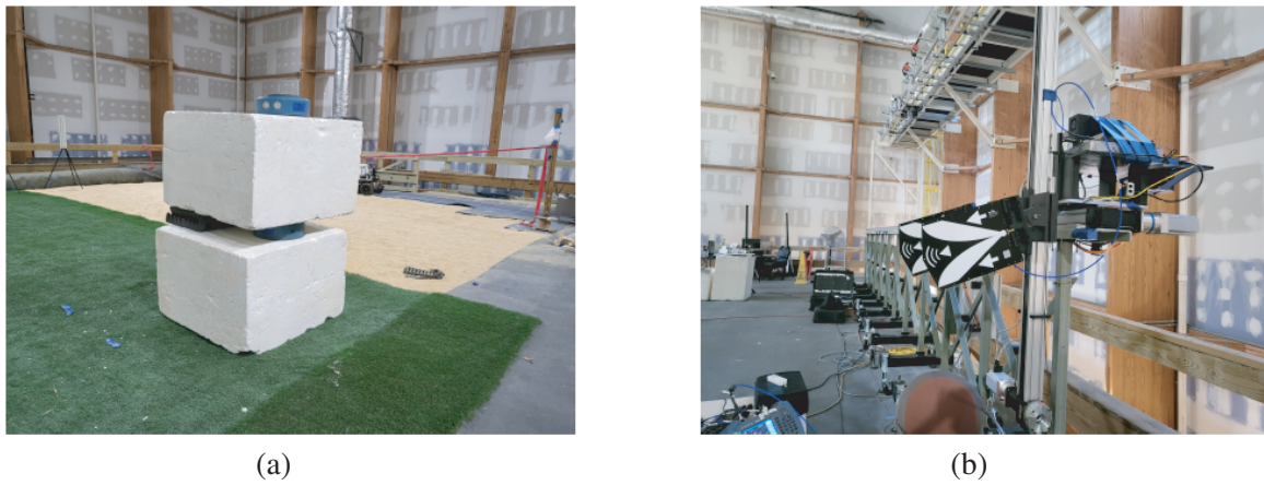
Figure 9. (a) Two landmines stacked vertically using styrofoam blocks. (b) Scanner on ARL facility capable of both vertical and horizontal scanning.
