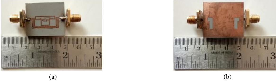
**Figure 9.** Fabricated notched band UWB filter, (a) top view, (b) bottom view.
