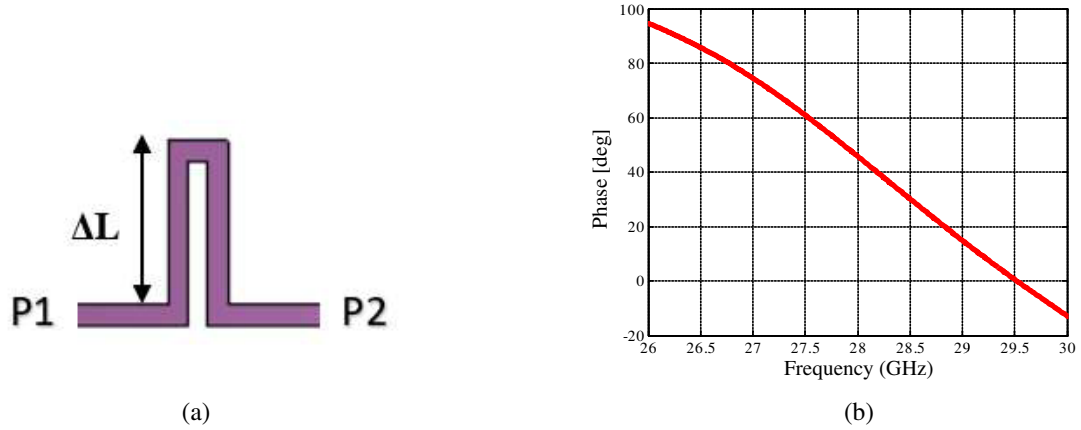
Figure 8. (a) Schematic diagram of a Phase shifter 45^\circ . (b) The Output Phase of Phase Shifter.
