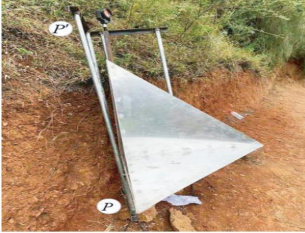
**Figure 8.** Experimental trihedral corner reflector device.
