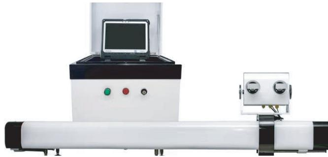
**Figure 7.** Micro Deformation Monitoring Radar LSA monitoring system.
