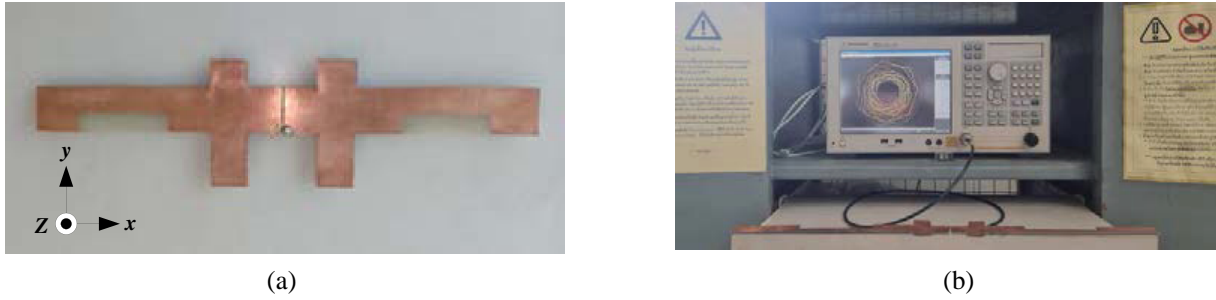
Figure 13. Photograph of proposed planar dipole antenna and equipment, (a) the prototype antenna was fabricated using the parameters in Table 1 and (b) Network Analyzer (Agilent: E5071C) was used to measure antenna characteristics.
