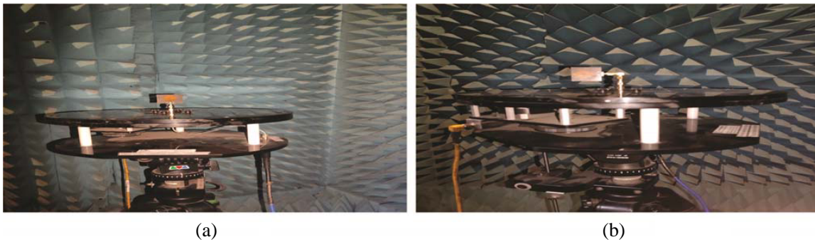
Figure 8. Radiation pattern measurement setup in anechoic chamber (a) E -plane, (b) H -plane.
