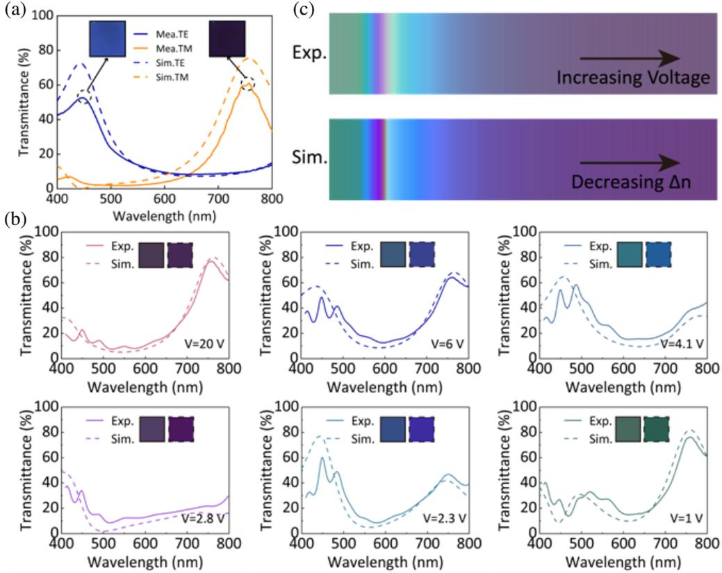
**Figure 3.** The color appearance and transmissive responses of the fabricated MFP filter. (a) The as-fabricated MFP without an LC cell. (b) The responses of the filter after integrating with an LC cell as the input voltage varies. (c) The simulated and measured colors as the phase retardation of the LC cell varies from  $2\pi$  to 0 (voltage from 0 to 20 V).
