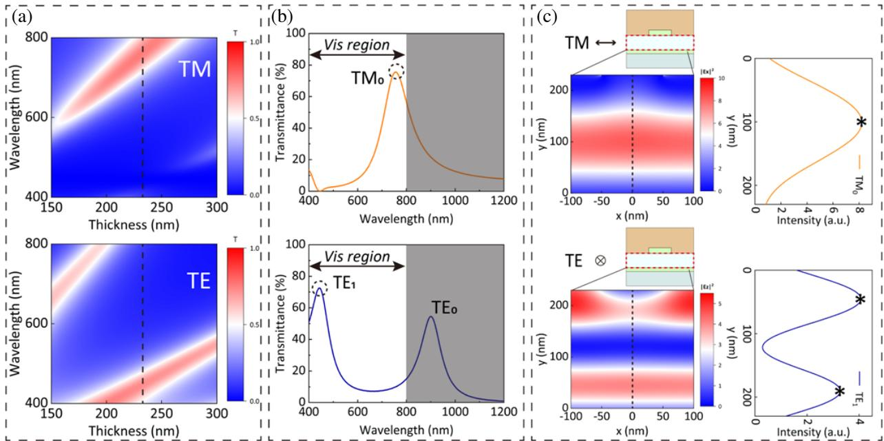
**Figure 2.** The simulation results for TE and TM input. (a) The response for TE and TM input with various insulator thicknesses. (b) The transmittance for TE and TM input for insulator thickness  $t = 230$  nm (dashed lines in Figure 2(a)). (c) The mode profiles in the cavity for the corresponding modes labeled in Figure 2(b) by dashed circles. The antinodes is labeled as asterisks.
