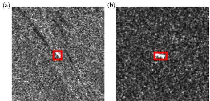
FIGURE 5. Ship detection results for SAR images.
