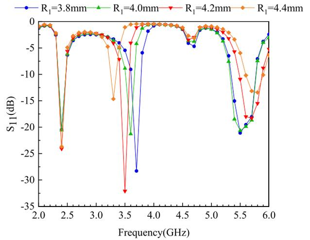
**Figure 19.** Effect of large elliptical diameter  $R_1$  on  $S$ -parameters.
