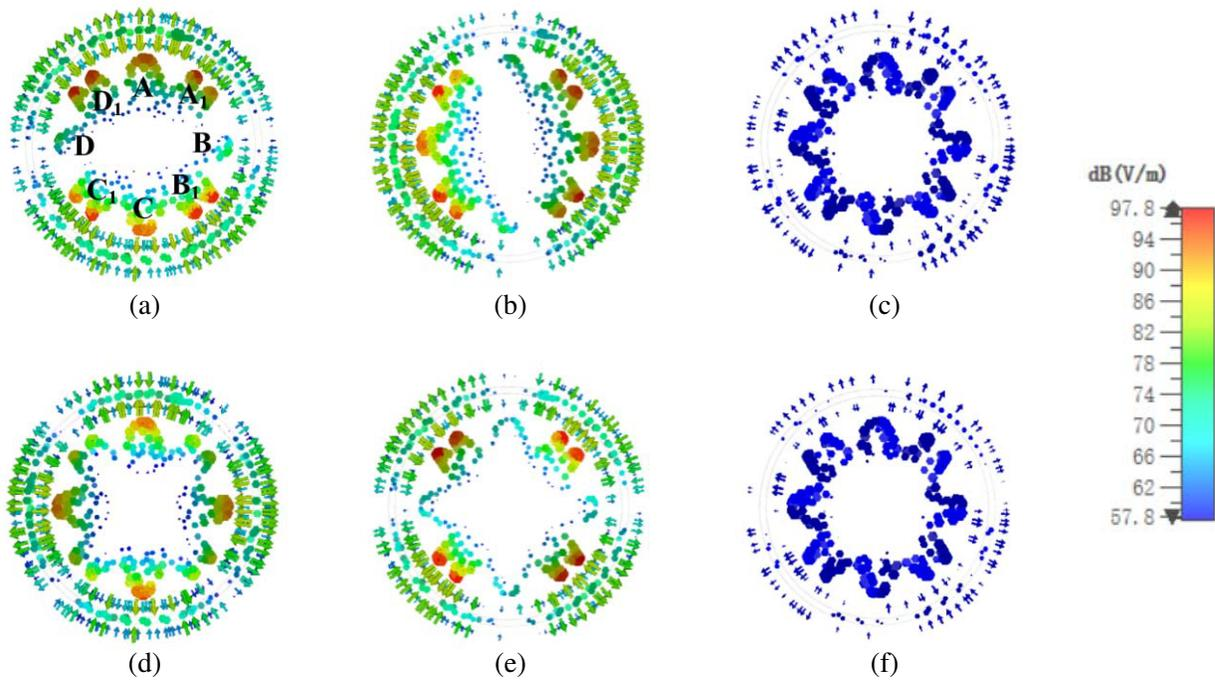
**Figure 5.** Electric field distribution of model I: (a) Mode 1 at 2.664 GHz; (b) Mode 2 at 2.664 GHz; (c) Mode 3 at 2.664 GHz; (d) Mode 5 at 5.256 GHz; (e) Mode 6 at 5.256 GHz; (f) Mode 3 at 5.256 GHz.
