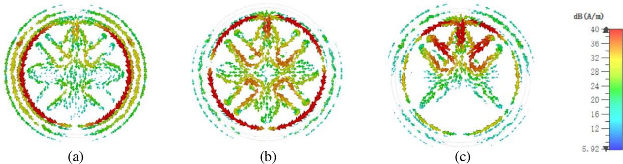
**Figure 13.** Current distribution at the MS resonance mode of interest: (a) Mode 1; (b) Mode 4; (c) Mode 11.
