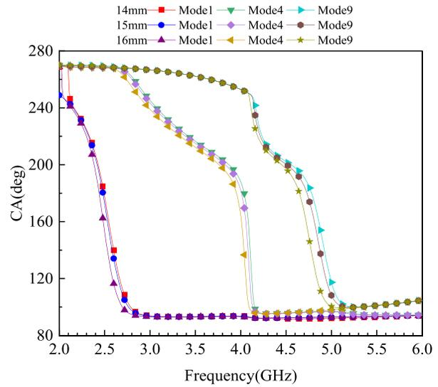
**Figure 10.** CA distribution of model III resonance modes at different  $R_7$ .
