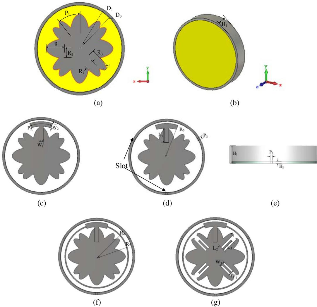
**Figure 1.** Antenna original model I: (a) Bottom view; (b) Side view; (c) Model II: Unslotted model; (d) Model II: Slotting model; (e) Side view model of slotting; (f) The proposed structural model III; (g) The proposed structural model IV.
