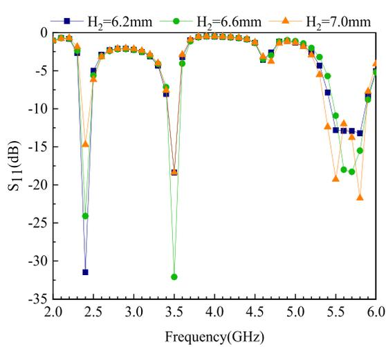
**Figure 18.** Effect of frame height  $H_2$  on  $S$ -parameters.
