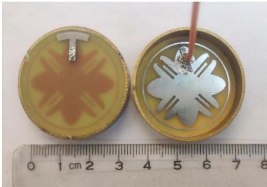
**Figure 14.** Front and back view of the proposed antenna.
