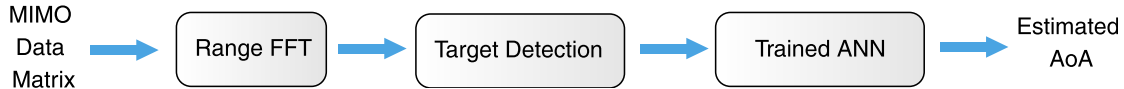
Figure 4. Data processing steps of the proposed method: 1) Range extraction through FFT along the fast-time axis. 2) Target detection. 3) DoA estimation with the trained neural network.
