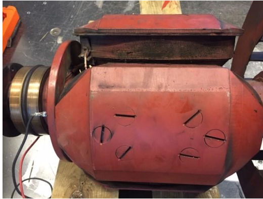
Figure 2. The test field winding of a four solid pole salient pole rotor.
