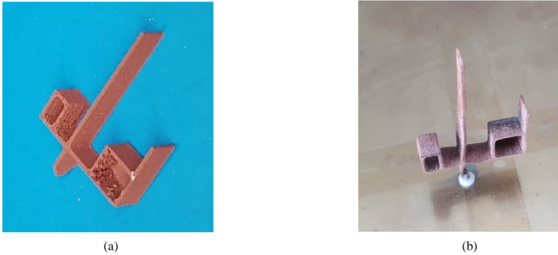
Figure 3. Manufactured antenna. (a) Composite material. (b) Sintered.
