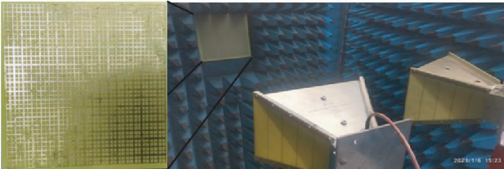
Figure 8. Measurement setup for proposed antenna.
