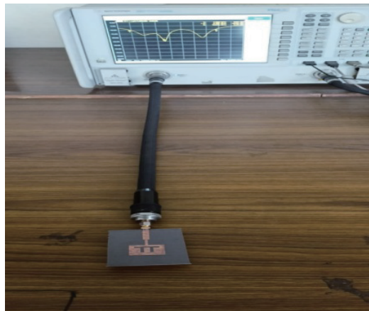
Figure 5. Experimental setup of proposed Pi-slot patch antenna with T-slot DGS.
