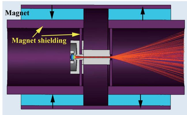
**Figure 13.** Diagram of the designed beam optics system.
