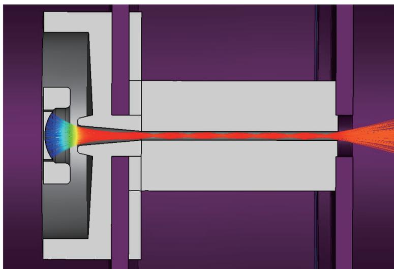
**Figure 15.** Trajectories of electrons.
