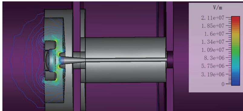
**Figure 16.** Electric field distribution in the gun area.
