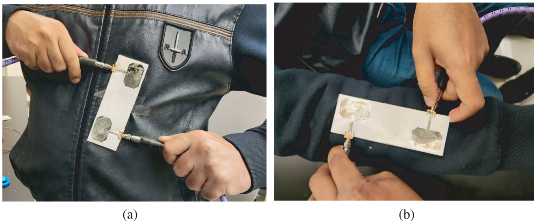
Figure 17. Proposed antenna tested on different parts of the body. (a) Belly. (b) Arm.
