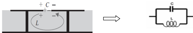
Figure 11. Typical Lumped LC model of EBG structure.
