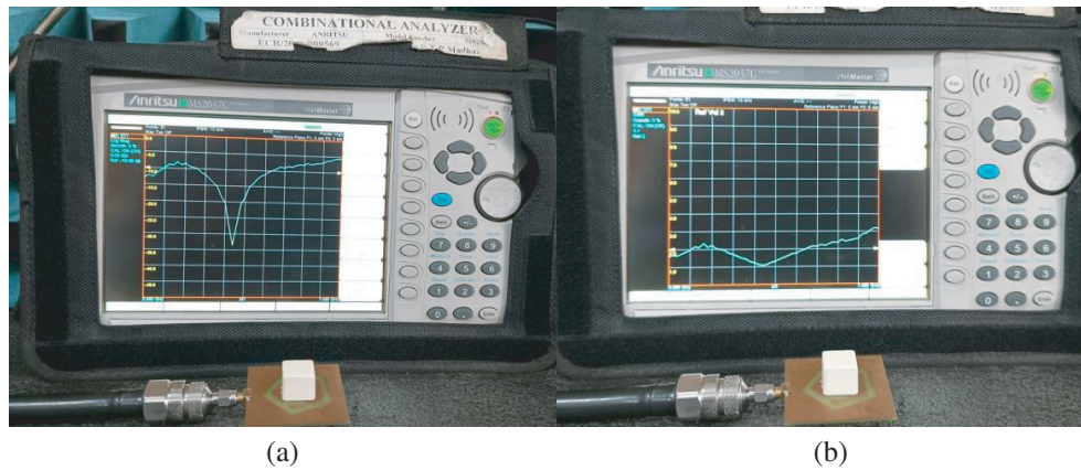
Figure 6. Pentagonal shaped DGS with RDRA. (a) Measurement setup for reflection coefficient. (b) Measurement setup for VSWR.
