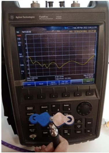
Figure 13. The connection of the fabricated antenna prototype to the VNA N9918A for measuring the reflection coefficient over the operating frequency band.
