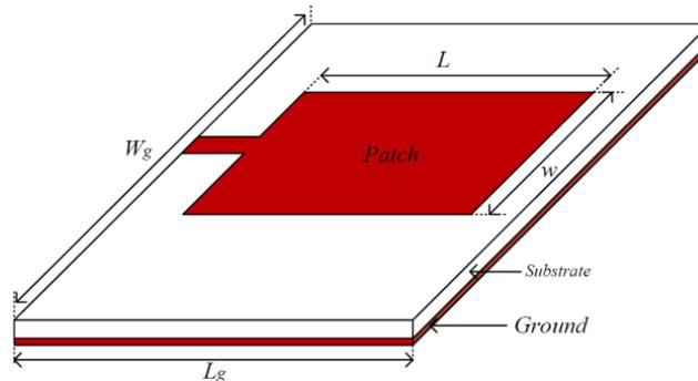
**Figure 1.** Configuration of a rectangular microstrip patch antenna.
