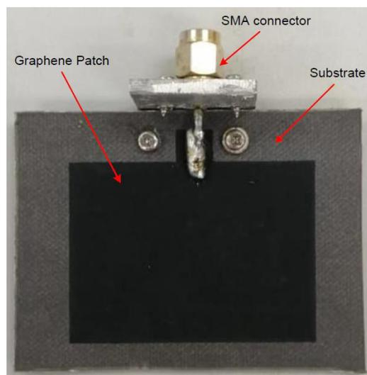
**Figure 4.** Fabricated graphene-based microstrip patch antenna.
