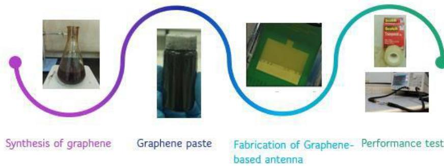
**Figure 3.** Graphical representation of graphene-based patch antenna fabrication.
