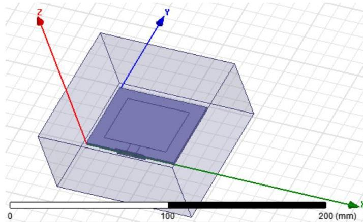
**Figure 2.** Patch antenna model from the HFSS-13 programme.
