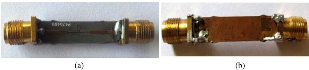
**Figure 13.** Photos of the fabricated prototype of the EBG-loaded BPF, (a) top-view, and (b) bottom-view.
