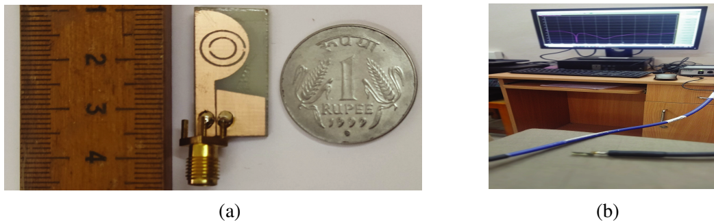
Figure 5. (a) Fabricated antenna. (b) Measurement setup.
