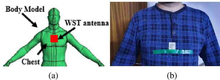
Figure 14. (a) Antenna on phantom body, (b) antenna mounted on human body.
