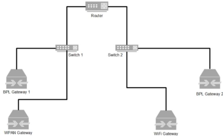
Figure 7. Typical architecture of a collapsed backbone network.
