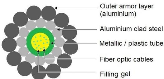
**Figure 1.** Typical cross section of an OPGW.
