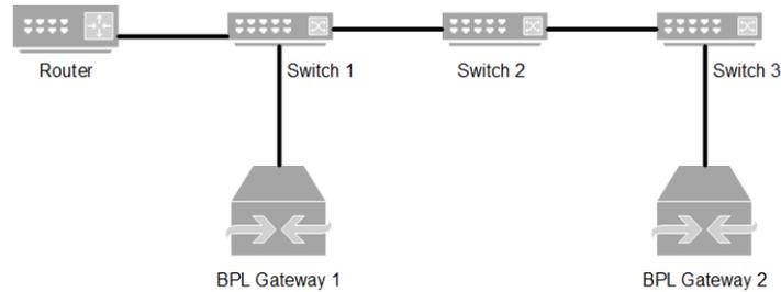
**Figure 5.** Typical architecture of a serial backbone network.
