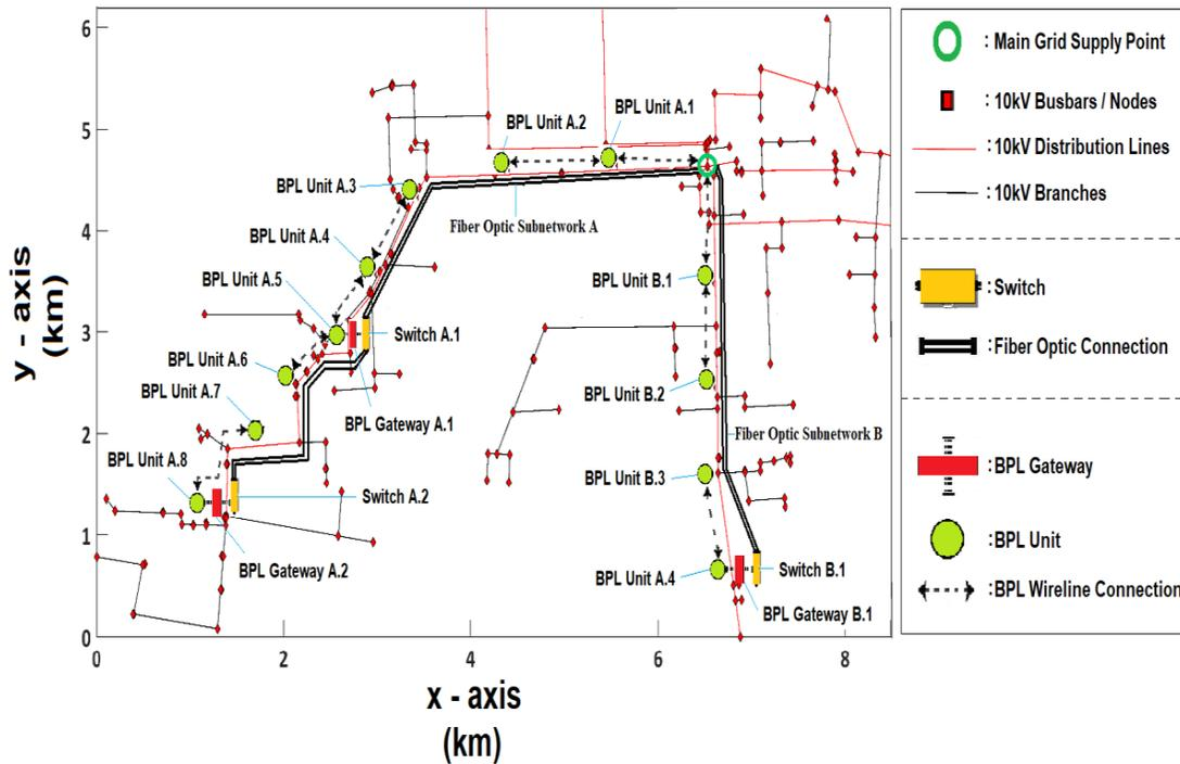
**Figure 14.** Theoretical field installation of a fiber optic backbone communications network and a BPL network across the real world overhead MV power grid of [72, 73].
