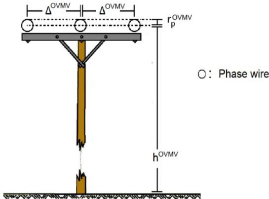
**Figure 10.** Typical overhead MV MTL configuration [23].
