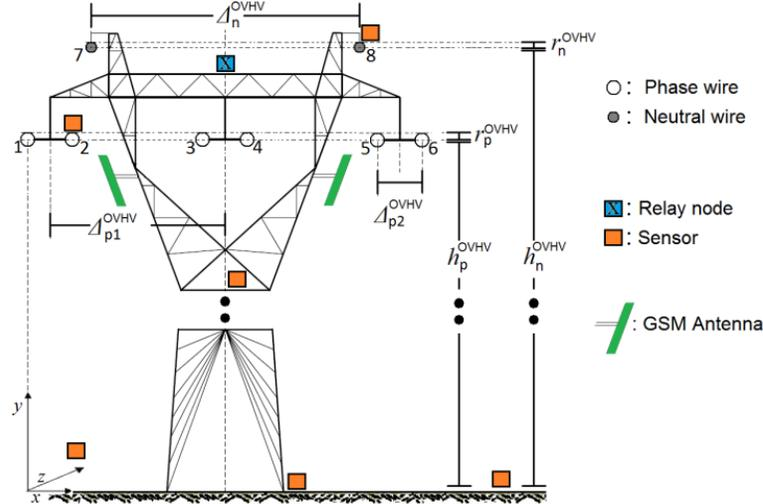
**Figure 9.** Typical overhead HV MTL configuration.
