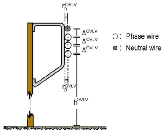
**Figure 11.** Typical overhead LV MTL configuration [23].
