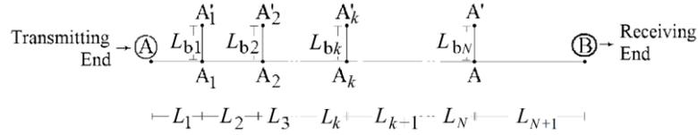
**Figure 12.** Typical overhead BPL topology with  $N$  branches [66].
