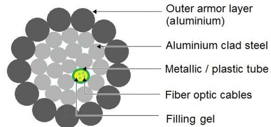
**Figure 2.** Typical cross section of an OPAC.
