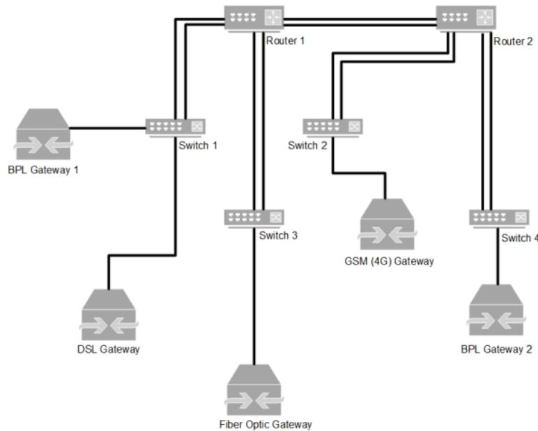
Figure 8. Typical architecture of a parallel backbone network.
