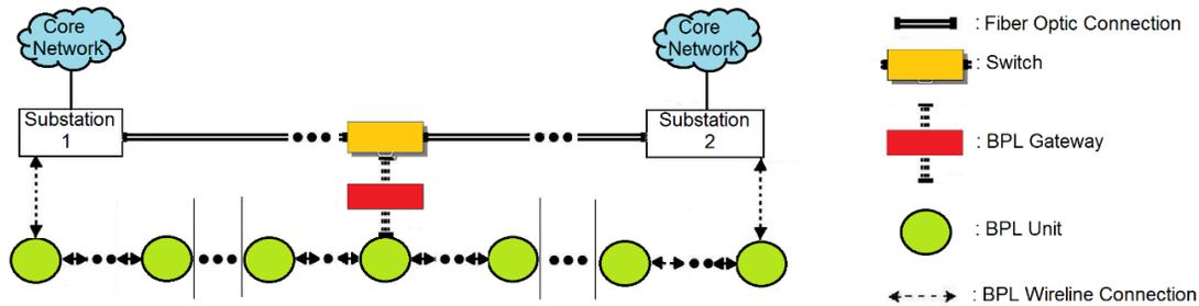
**Figure 13.** Overhead transmission and distribution BPL network model for the connection with the fiber optic backbone communications network through BPL gateways.
