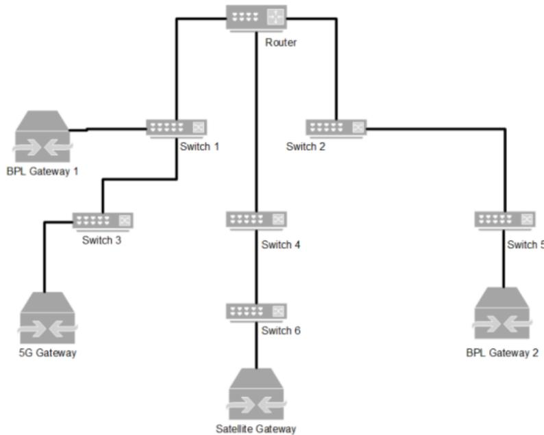
**Figure 6.** Typical architecture of a distributed backbone network.
