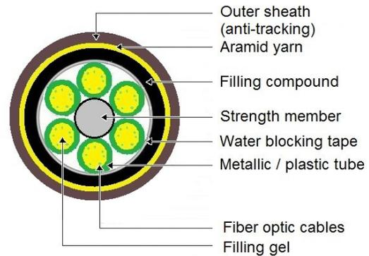
**Figure 3.** Typical cross section of an ADSS wire.
