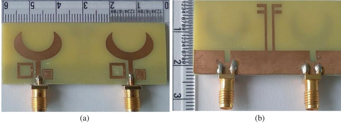
**Figure 11.** Fabricated antenna. (a) Patch. (b) Ground.
