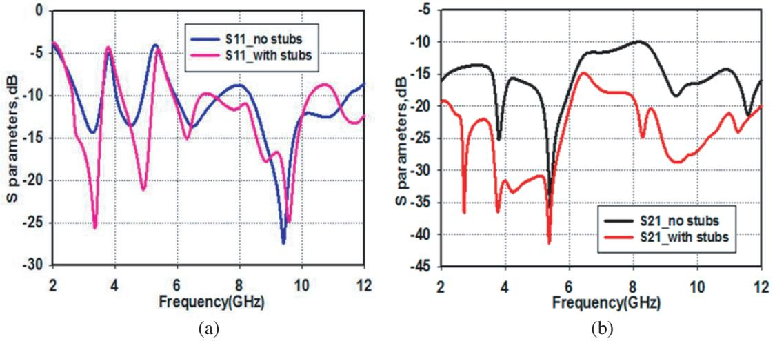
Figure 8.  $S$  parameters, (a)  $S_{11}$ , (b)  $S_{21}$ .
