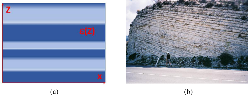
Figure 1. Geometry of the problem of interest. (a) The dielectric permittivity \varepsilon(z) of a bulk conductive medium is continuous and depends only on z coordinate, which is illustrated by halftones. In a strongly lossy conductive medium the dielectric permittivity is almost pure imaginary: \varepsilon(z) \approx i\varepsilon''(z) = i\sigma(z)/\varepsilon_0\omega . (b) Example of a conductive layered sedimentary rock.
