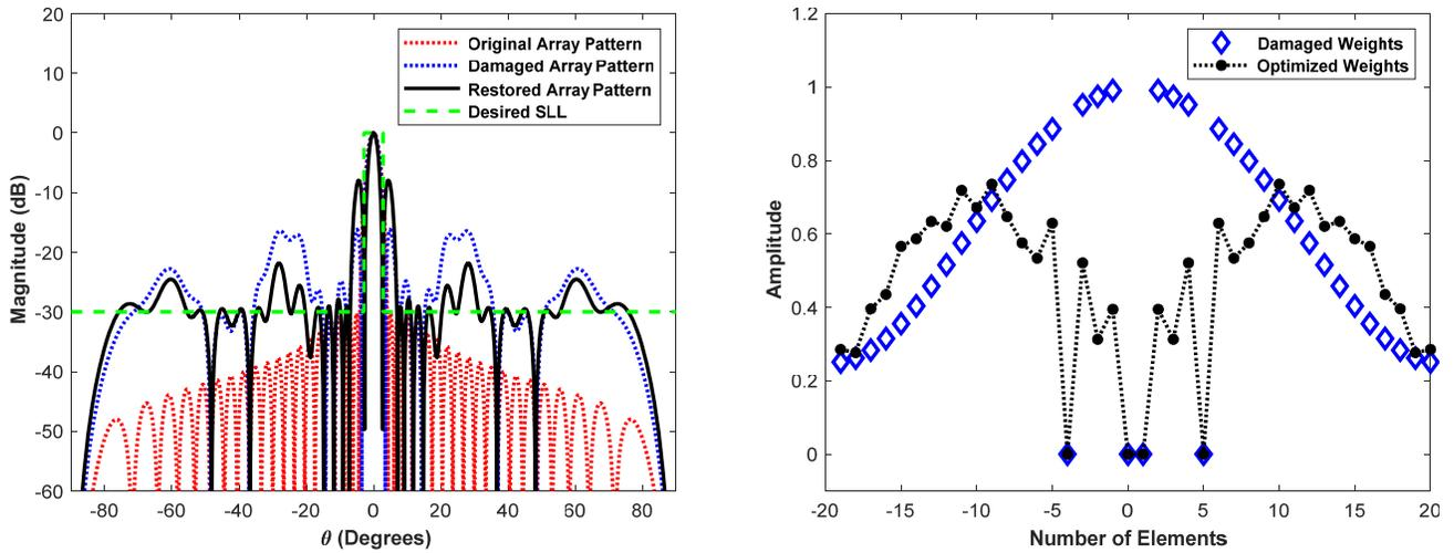
**Figure 7.** The original, damaged and the restored array patterns and their corresponding amplitude weights for 4 defective elements at the array center.
