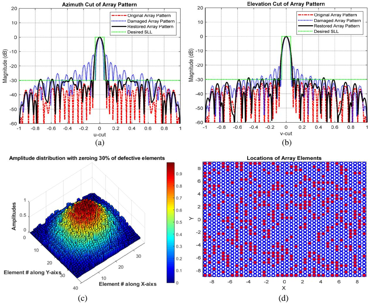
**Figure 9.** The original, damaged and the restored array patterns for (a) azimuth plane, (b) elevation plane, their amplitude weights with (c) 30% randomly defective elements, and (d) defective element locations highlighted in red color.
