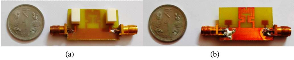
**Figure 9.** Fabricated prototype of the designed antenna. (a) Top view. (b) Back view.
