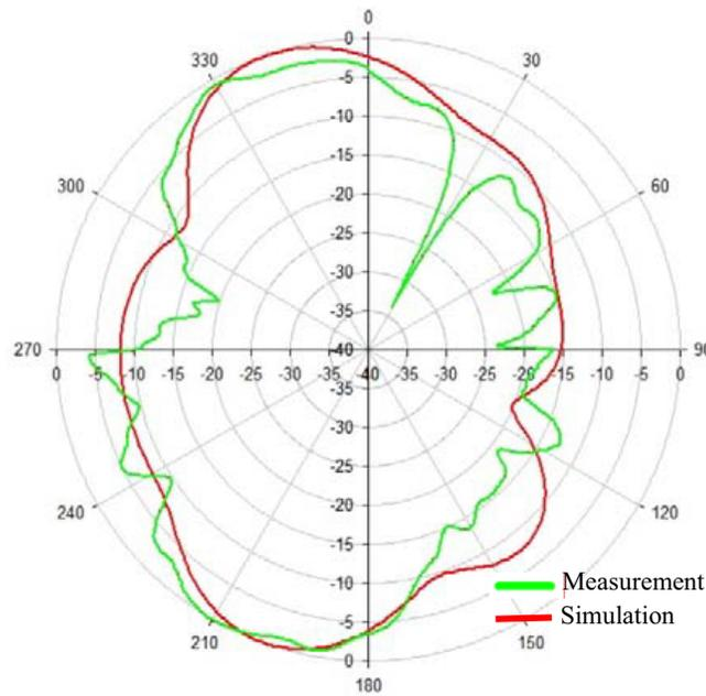
Figure 12. Radiation pattern for simulation and measurement.
