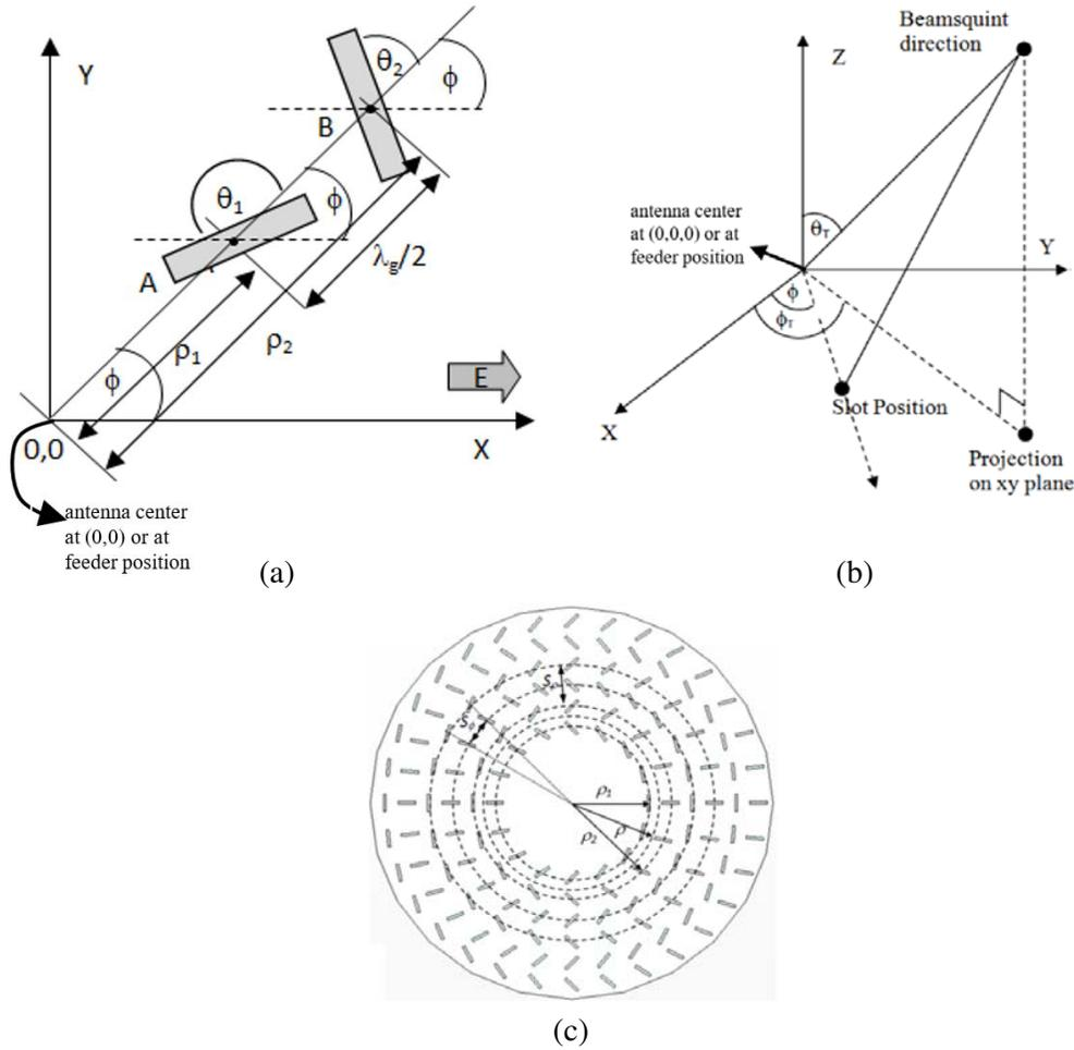
**Figure 2.** (a) Parameters of slots in the  $x$ - $y$  plane, (b) slots' positions and their relationships in respect to the beam direction in  $x$ - $y$ - $z$ , and (c) distance between the slots in radial and azimuth directions [15].
