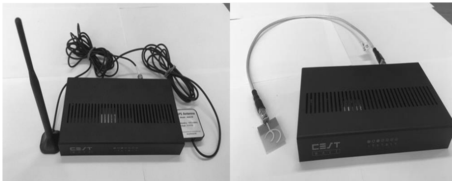
Figure 10. Coupling test setup using vehicular communication module.
