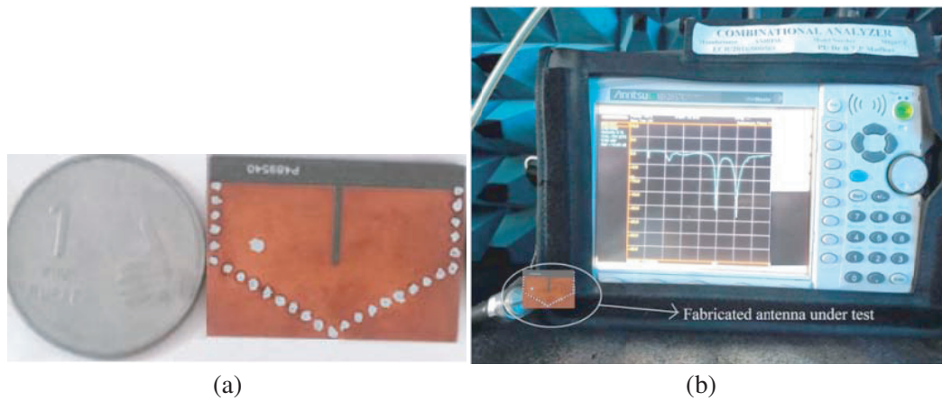
Figure 9. (a) Top View of the Proposed Antenna prototype, (b) S_{11} measurement setup of proposed antenna.
