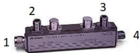
Figure 2. Hewlett Packard 777D 1.9–4 GHz with -20 dB coupling factor. ‘1’ represents the input port, ‘2’ represents the forward coupled port, ‘3’ represents the reverse coupled port, and ‘4’ represents the output port. (Figure obtained from www.keysight.com ).
