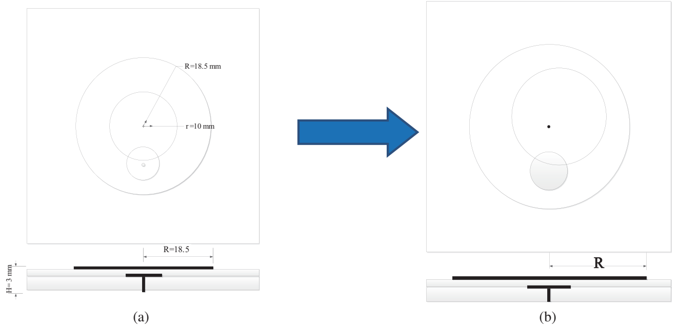
Figure 6. Antenna circular polarization design concept. (a) Antenna II structure diagram. (b) Antenna III structure diagram.
