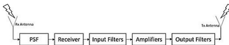
Figure 1. Simplified block diagram of satellite signal chain.
