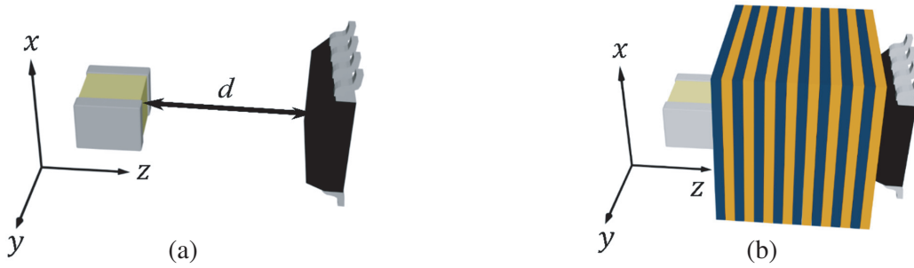
Figure 1. (a) Two objects are placed at a distance d in z direction. (b) Alternating layers of two materials form a NUM between the two objects.
