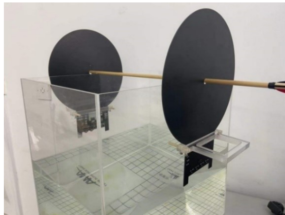
Figure 11. Experimental system for underwater wireless power transmission.
