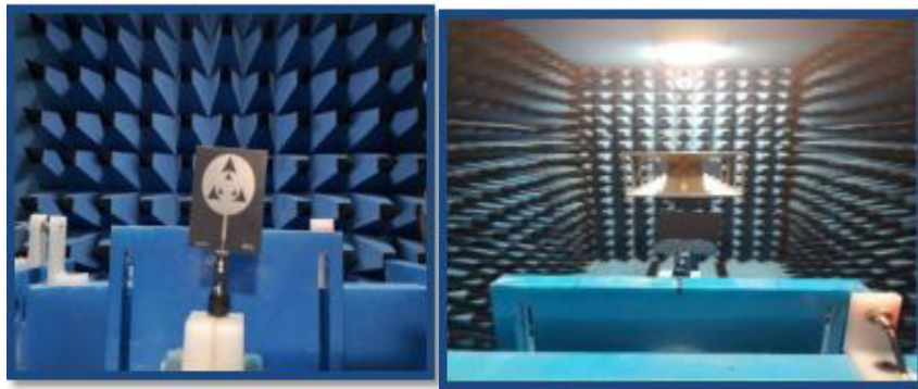
Figure 16. Measurement set up of proposed antenna in anechoic chamber.
