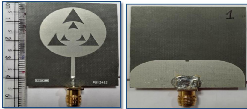
Figure 15. Front and back side of fabricated patch antenna.
