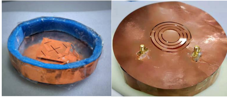
Figure 3. Fabricated cavity-enclosing patch antenna.
