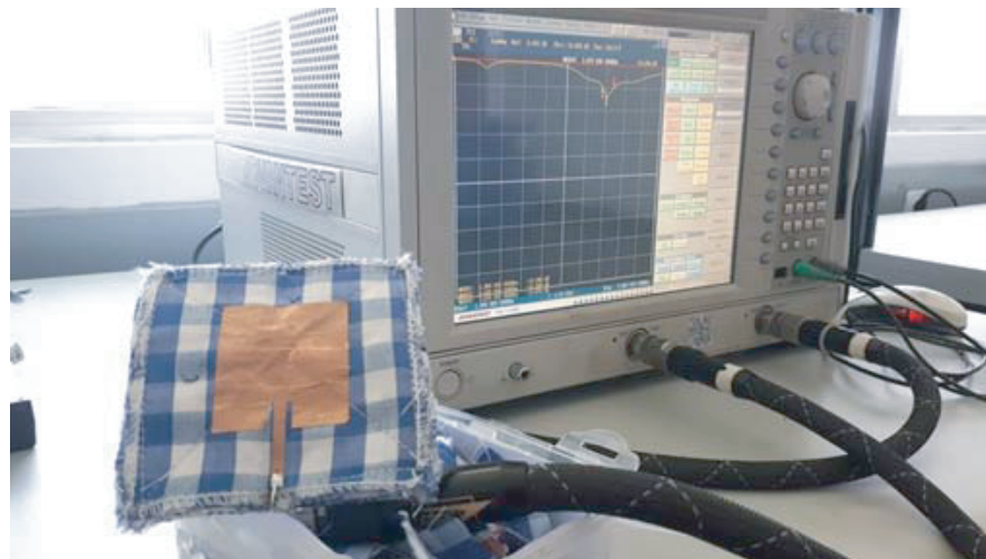
Figure 7. The measurement of the proposed antenna wearable.
